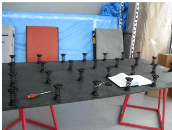
Figure 1. Spring configuration on the underside of a spring-floor fiberglass wood laminate panel.
