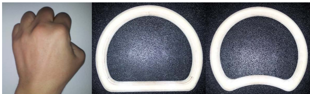
Figure 2. a - palm grasp, b – rings with straight part, c – rings with bent part inward
